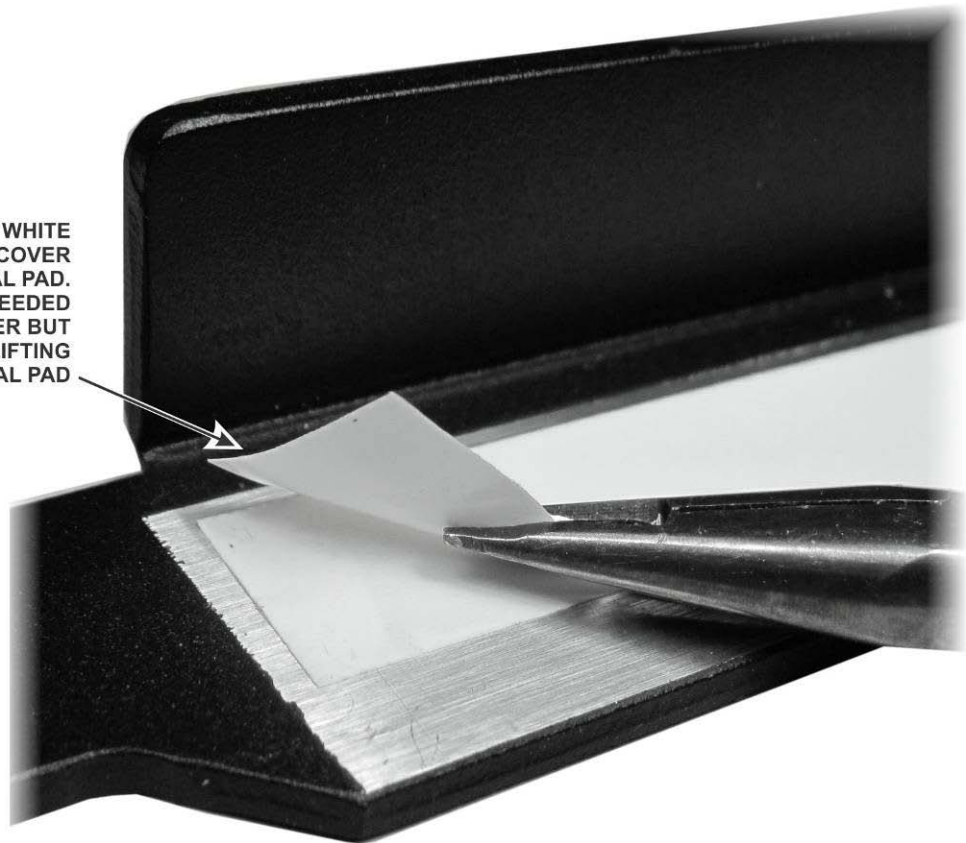
Figure 40. Removing the Clear Plastic Protective Cover from the Heat Sink.
