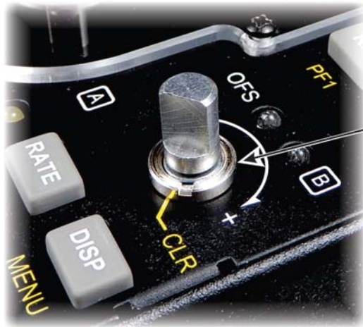
Figure 17. Mounting the Ring Nut on the VFO B Encoder.
