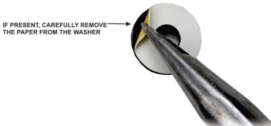
Figure 14. Preparing the Rubber Washer for Mounting on the VFO B Encoder.
