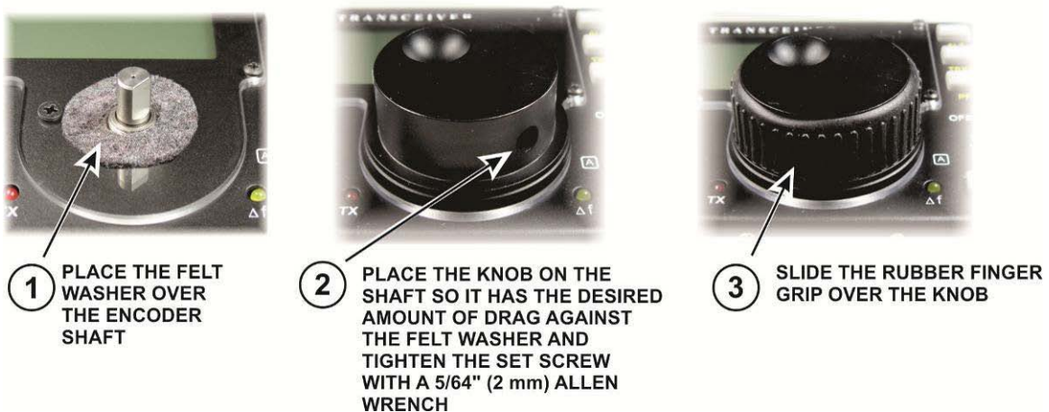
Figure 23. Mounting the VFO Knob.
